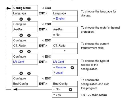
\* No transformation ratio is saved in the factory settings. This parameter must be entered before you can exit the **Config Menu** program.
